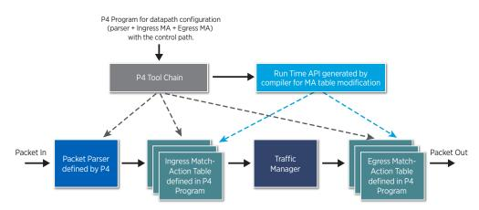
The SDK supports P4 syntax as defined on the P4 specifications published on P4 consortium website (www.p4.org). Corigine has integrated the open source P4 compiler in the SDK generate an intermediate representation (App.IR) of the P4 program in the yaml format, which is further compiled by the P4 back-end compiler to generate a C program for the data path on the NFP. P4 programming support on the SDK is shown in the figure below.
