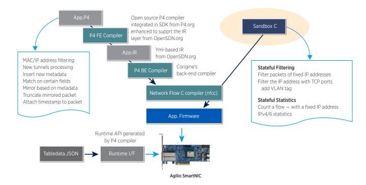
Since P4 is meant for hardware independent programming (flow processing), the user does
